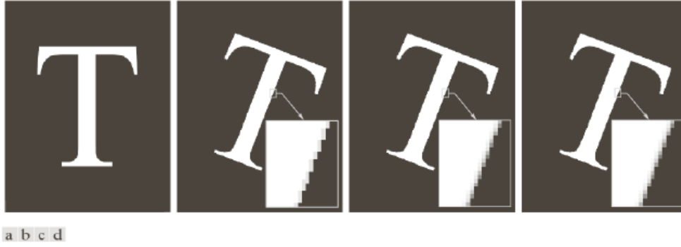
FIGURE 2.36 (a) A 300 dpi image of the letter T. (b) Image rotated 21° clockwise using nearest neighbor interpolation to assign intensity values to the spatially transformed pixels. (c) Image rotated 21° using bilinear interpolation. (d) Image rotated 21° using bicubic interpolation. The enlarged sections show edge detail for the three interpolation approaches.
