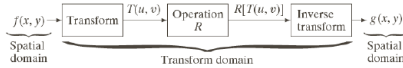
FIGURE 2.39 General approach for operating in the linear transform domain.
