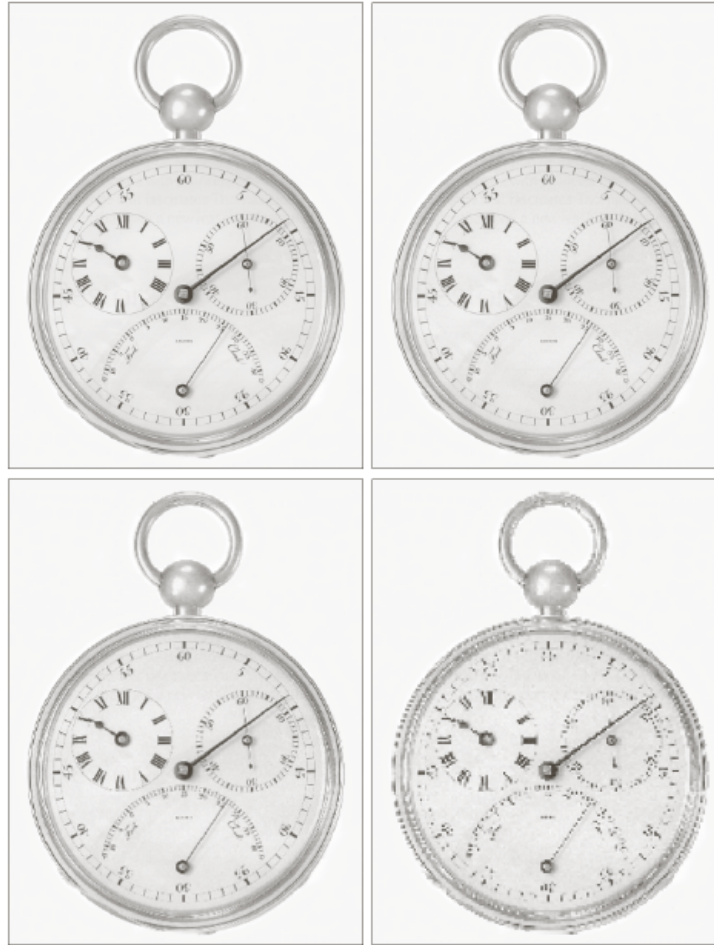
FIGURE 2.20 Typical effects of reducing spatial resolution. Images shown at: (a) 1250 dpi, (b) 300 dpi, (c) 150 dpi, and (d) 72 dpi. The thin black borders were added for clarity. They are not part of the data.
