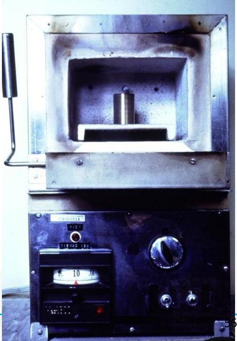
Place ring in oven with hole down. Be sure to remove sprue former first.
