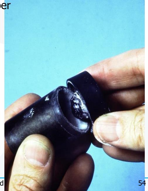
Inspect for defects-voids and positives
